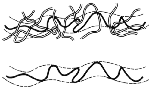
Figure 21. Reptation of a test chain (black) through the segments of a matrix (white). The “walls” of the tube are indicated by dotted lines.
